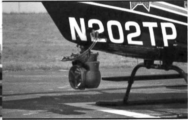
FIGURE 3 – THE HSL-1600 ON A BELL 206
