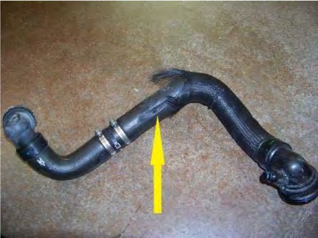
LOWER RADIATOR HOSE WORE THROUGH DUE TO CONTACT WITH A/C COMPRESSOR (9,863 TEST MILES)
