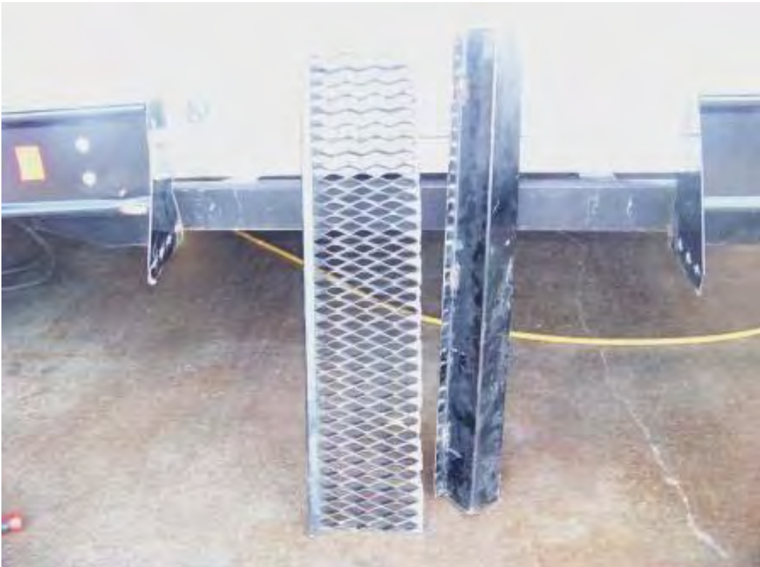
REAR BUMPER STEP BROKEN OFF (2,273 TEST MILES)
