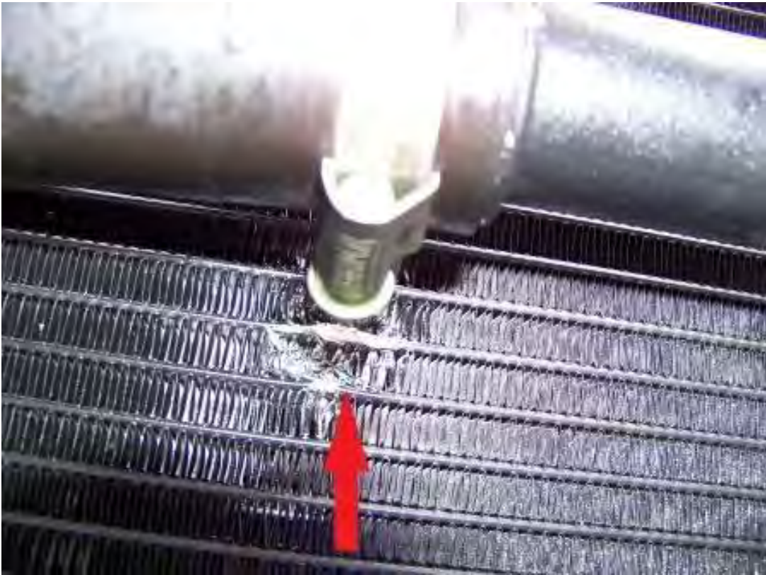
CLAMP RUBBING THROUGH A/C CONDENSOR (1,528 TEST MILES)
