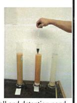
There will be additional detailed testing for the outfall and detention pond and erosion protection. These tests will consist of crumb tests and double hydrometer tests to evaluate the dispersive characteristics of the on-site soils.
