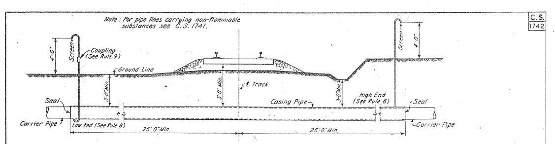
RULES GOVERNING\_THE INSTALLATION OF PIPE LINES TRANSMITTING FLAMMABLE SUBSTANCES WHEN CROSSING UNDER TRACKS: GENERAL.
