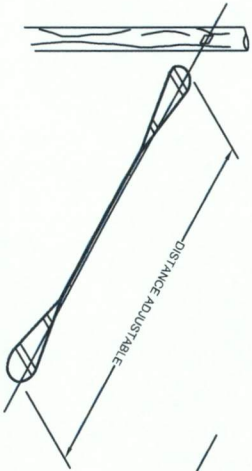
TYPICAL DETAIL "A" RESERVE CABLE LENGTH STRAND STORAGE APPLICATION
