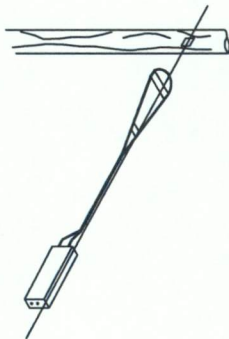
TYPICAL DETAIL "C" BUTT SPLICE APPLICATION
