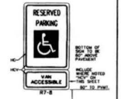
TYPICAL HANDICAP PARKING SIGN DETAIL
