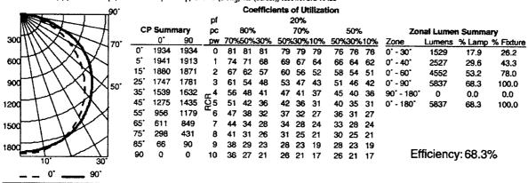
2AV G 3 32 MDR ASR, (3) 32W T8 lamps, 2850 lumens per lamp, s/m 1.2 (along) 1.3 (across), test no. LTL 10120
