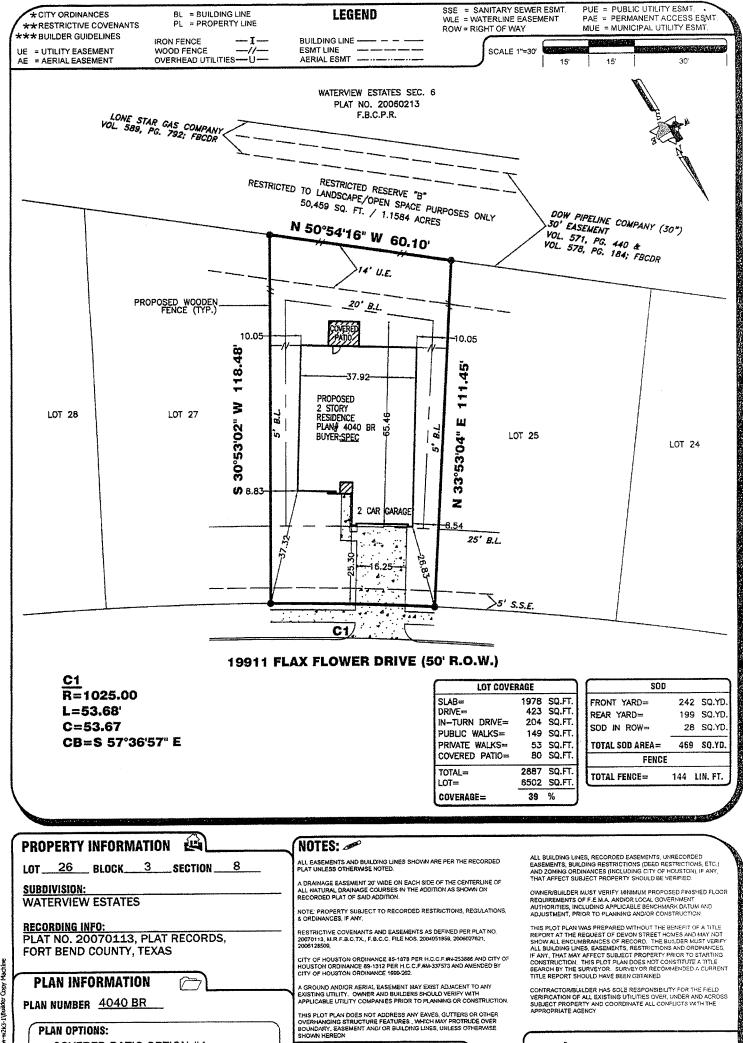
**PLAN OPTIONS:** -COVERED PATIO OPTION #1 FLOOD INFORMATION F.I.R.M. NO: <u>48157C</u> REVISED DATE: <u>01-03-97</u> PANEL: 0115J ZONE: "X" FLOOD INFORMATION PROVIDED HEREON IS BASED ON SCALING THE LOCATION OF THE SUBJECT TRACT ON THE FLOOD INSURANCE RATE MAPS. THE INFORMATION SHOULD BE USED TO DETERMINE FLOOD INSURANCE RATES ONLY AND IS NOT INTENDED TO IDENTIFY SPECIFIC FLOODING CONDITIONS. WE ARE NOT RESPONSIBLE FOR THE F.I.R.M.'S ACCURACY.
