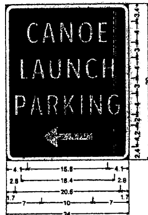
1.5" Radius, 0.8" Border, White on Brown; "CANOE" ClearviewHwy-2-W; "LAUNCH" ClearviewHwy-2-W; "PARKING" ClearviewHwy-2-W; Standard Arrow Custom 10.0" X 4.1" 180°;
