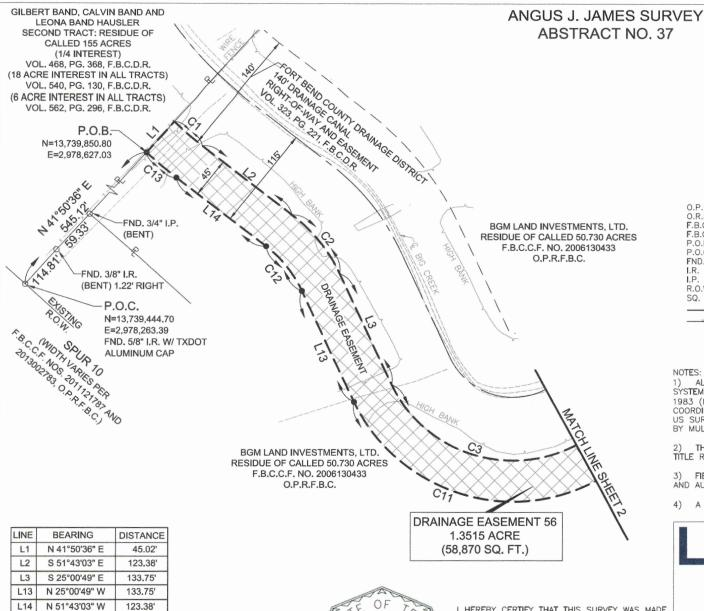
CURVE RADIUS LENGTH DELTA CHORD C1 420.00' 39.84 05°26'08" S 48°59'59" E 39.83 C2 180,00' 26°42'14" 83.14' 83.89 S 38°21'56" E C3 145,00' 267,15' 105°33'46" S 77°47'42" E 230.94 C11 190.00' 350.06 105°33'46' N 77°47'42" W 302.61 C12 135.00' 62,92 26°42'14" N 38°21'56" W 62.35 C13 465.00' 42.64 05°15'15" N 49°05'26" W 42.63
