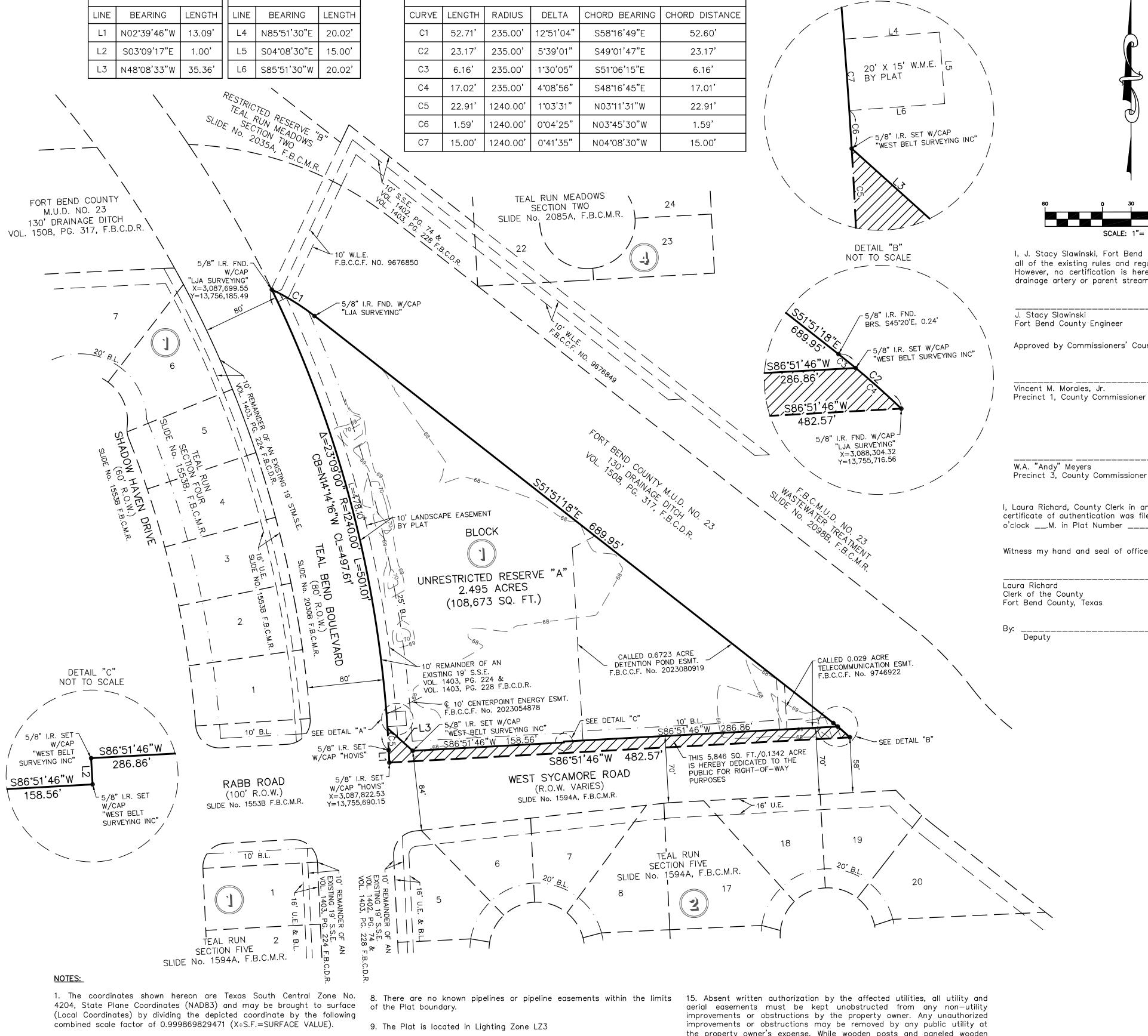
2. Bearings depicted hereon are based on Texas State Plane Coordinate System, South Central Zone (NAD83).
