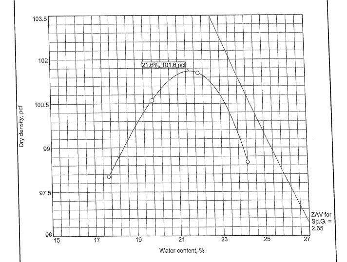
Test specification: ASTM D 698-12 Method A Standard
