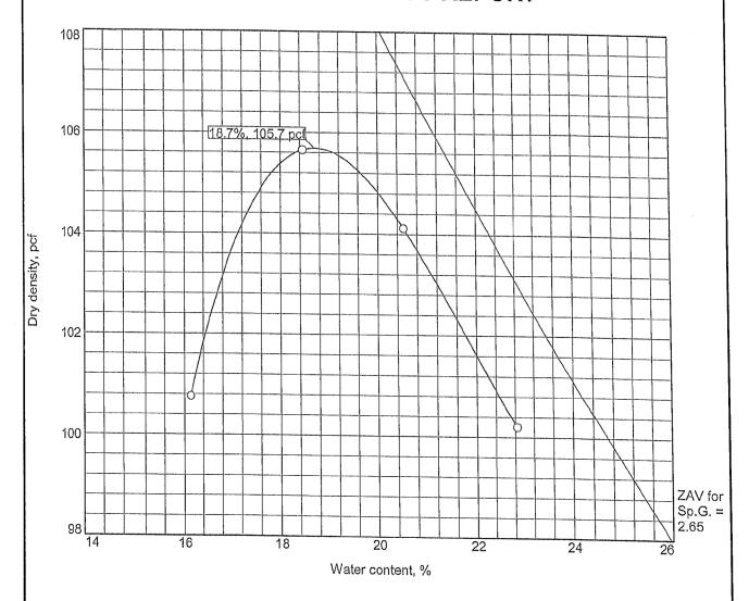
Test specification: ASTM D 698-12 Method A Standard
