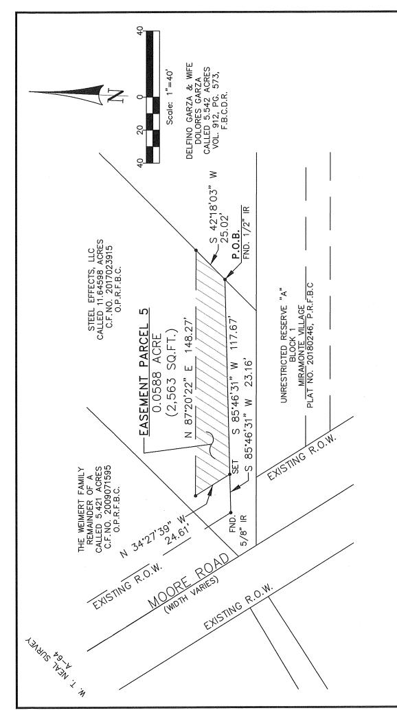
Bearings are based on the Texas Coordinate System of 1983, South Central This survey was performed without the benefit of at tile commitment, easements, coverants and/or restrictions may exist which are not shown hereon.
