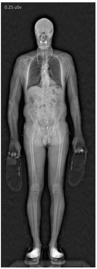
A typical image from Intercept on the lowest setting, 0.25 uSv. Items: teeth fillings, neck chain, object in shoe heal, ring and zipper. Intercept can operate at up to 200 uRem for even better image quality.
