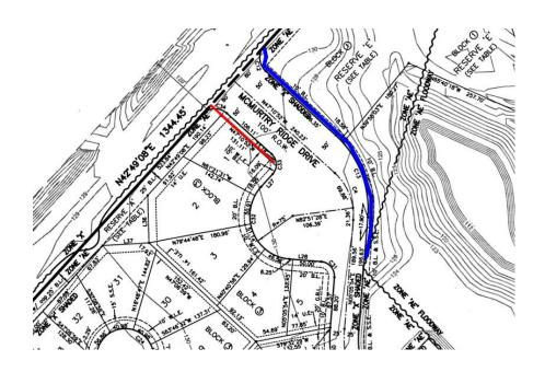
Due to the existing landscaping present in the area shown in red and in the image below, it is the hope of the Engineer and Developer that sidewalk construction will not be required. Sidewalk on the East side of McMurtry Ridge Drive will be constructed and there will be sidewalk access to Katy Flewellen Road.
