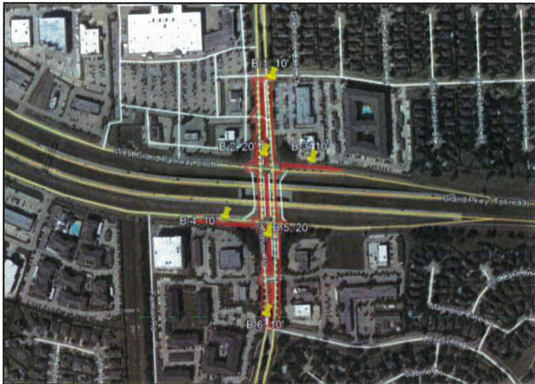
Plate 2 – Widening Plan of Mason Road at Texas State Highway 99 in Fort Bend County, Texas
