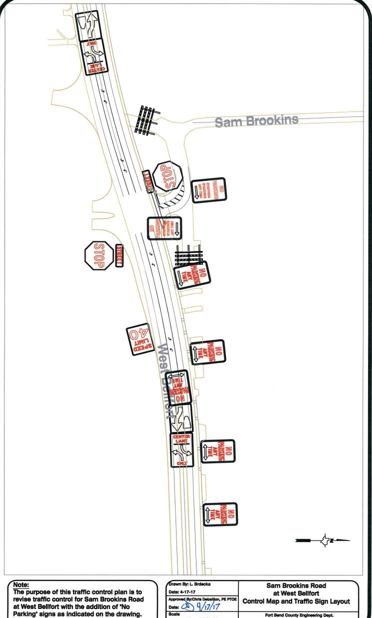
revise traffic control for Sam Brookins Road at West Bellfort with the addition of "No Parking" signs as indicated on the drawing.
