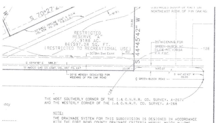
THE DRAINAGE SYSTEM FOR THIS SUBDIVISION IS DESIGNED IN ACCORDANCE WITH THE FORT BEND COUNTY DRAINAGE CRITERIA MANUAL WHICH ALLOWS STREET PONDING WITH INTENSE RAINFALL EVENTS.
